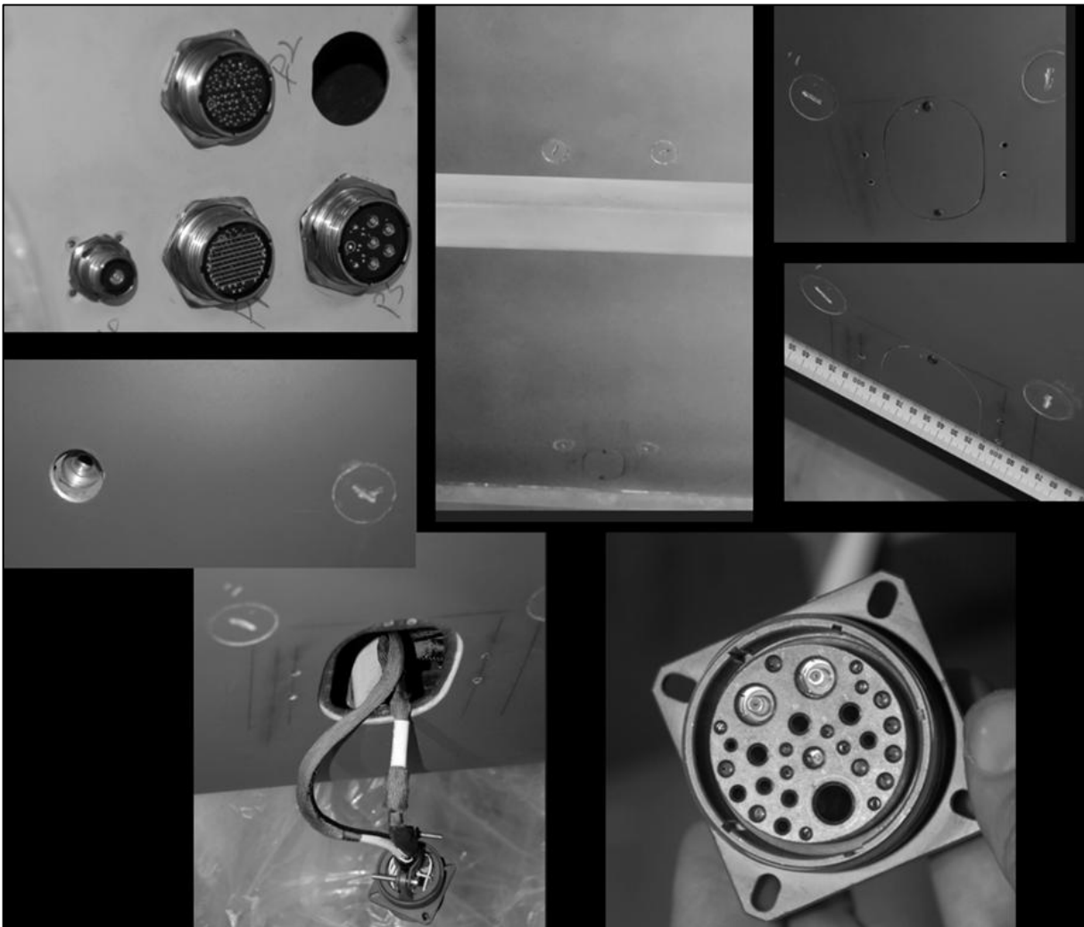
Figure 35.5 Wing cable connectors (top left); hard points for pylons with cabling
