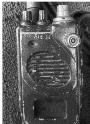
Close-up view of the Tadiran RT-7106 (PRC-710) control panel, showing selector knobs for CLR/SEC/AJ (Clear, Secure, Anti-Jamming) communication modes and an intact display window. The markings and wear indicate active operational deployment and prolonged field handling.
