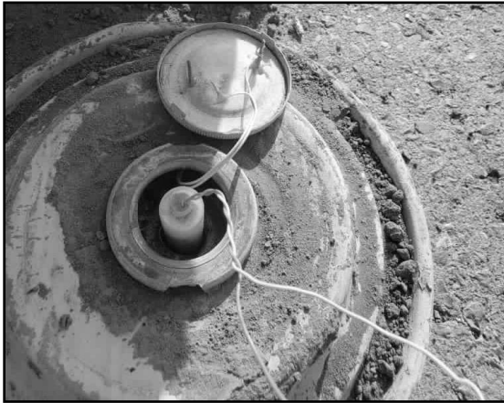
Figure 89.2.16 Improvised anti-tamper switch.
