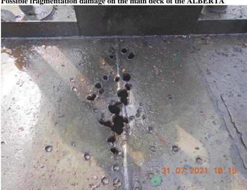
Figure 14.1 **Possible fragmentation damage on the main deck of the ALBERTA**
