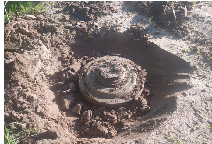
A TM-62M anti-vehicle mine equipped with MVCh-62 pressure activated fuze cleared near Kyivka in Chernihiv region, Ukraine, after a tractor driver was killed by another TM-62 mine in the same field on May 23, 2022. © 2022 State Emergency Services Facebook post
