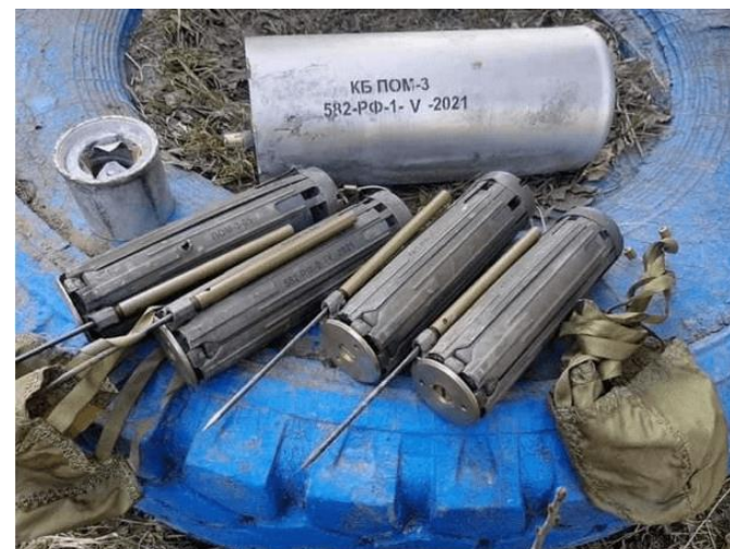
Four POM-3 antipersonnel mines that failed to deploy correctly and their dispenser found by deminers in the Kharkiv region, Ukraine, March 2022. © 2022 Private
