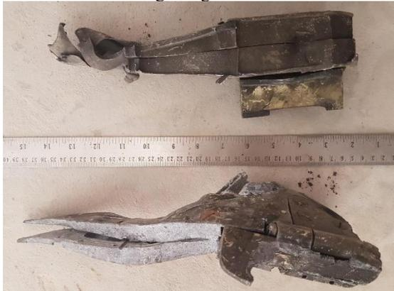
Compressor of a TRI-60 Microturbo engine
