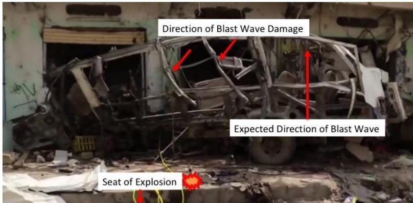
22. The final position of the bus requires further investigation and explanation. It is possible that it could have been thrown towards the shop front (marked B in figure 33.F.12) dependent on its position relative to the centre of the explosion. If the vehicle had been travelling in the normal position on the road, then it is more likely that the explosion would have projected it to position marked A in figure 30.F.12.
