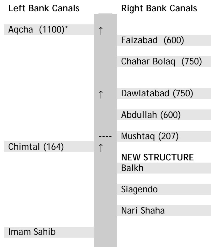
Figure 1: Schematic representation of canal structure of the Hazdha Nahr system
