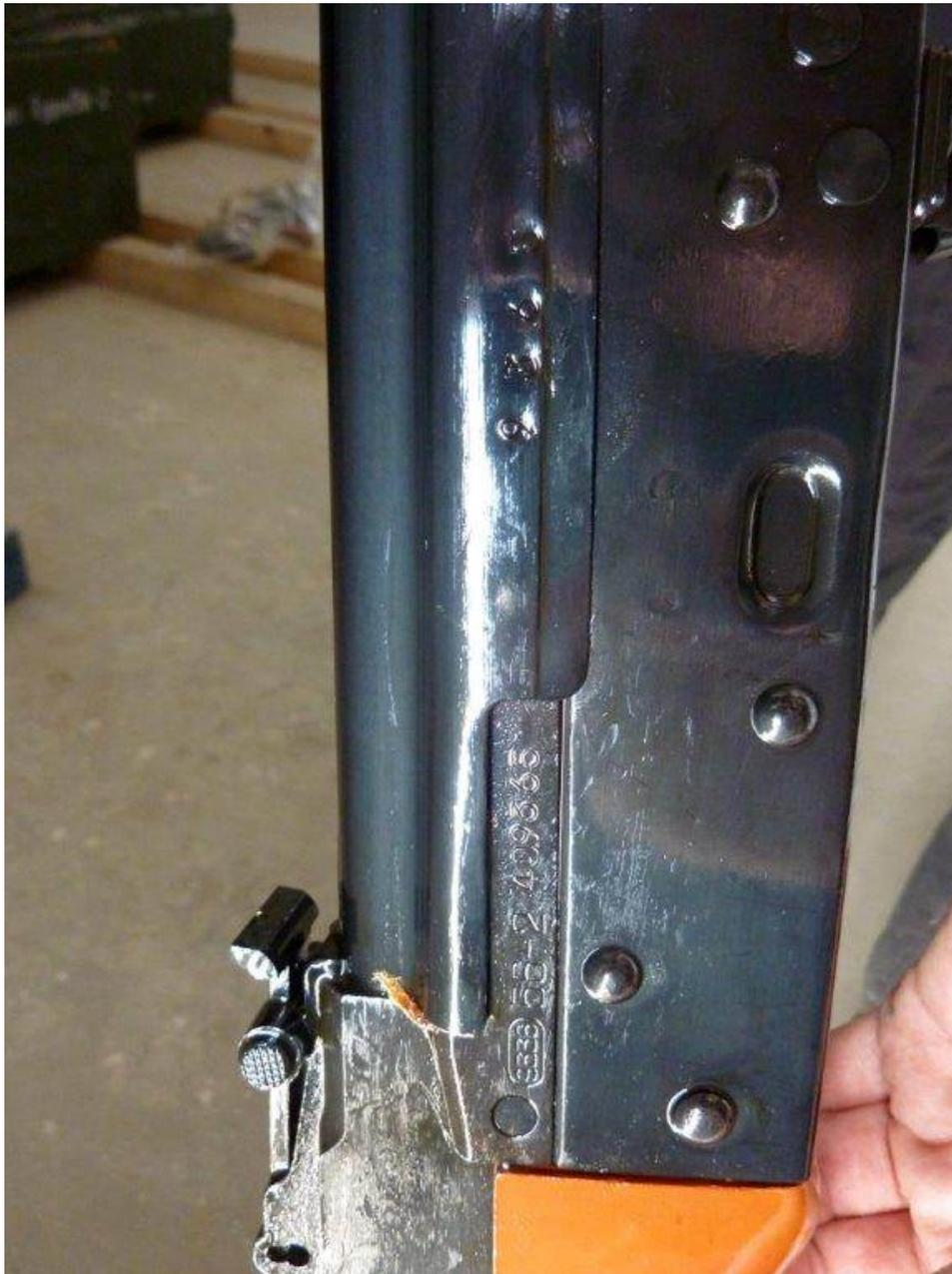
*Another sample of a rifle showing factory marking 386, type (56-2), and serial number with sequence beginning with "60"*
