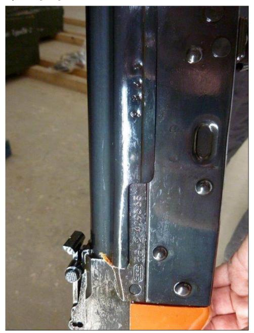
Another sample of a rifle showing factory marking 386, type (56-2), and serial number with sequence beginning with "60"
